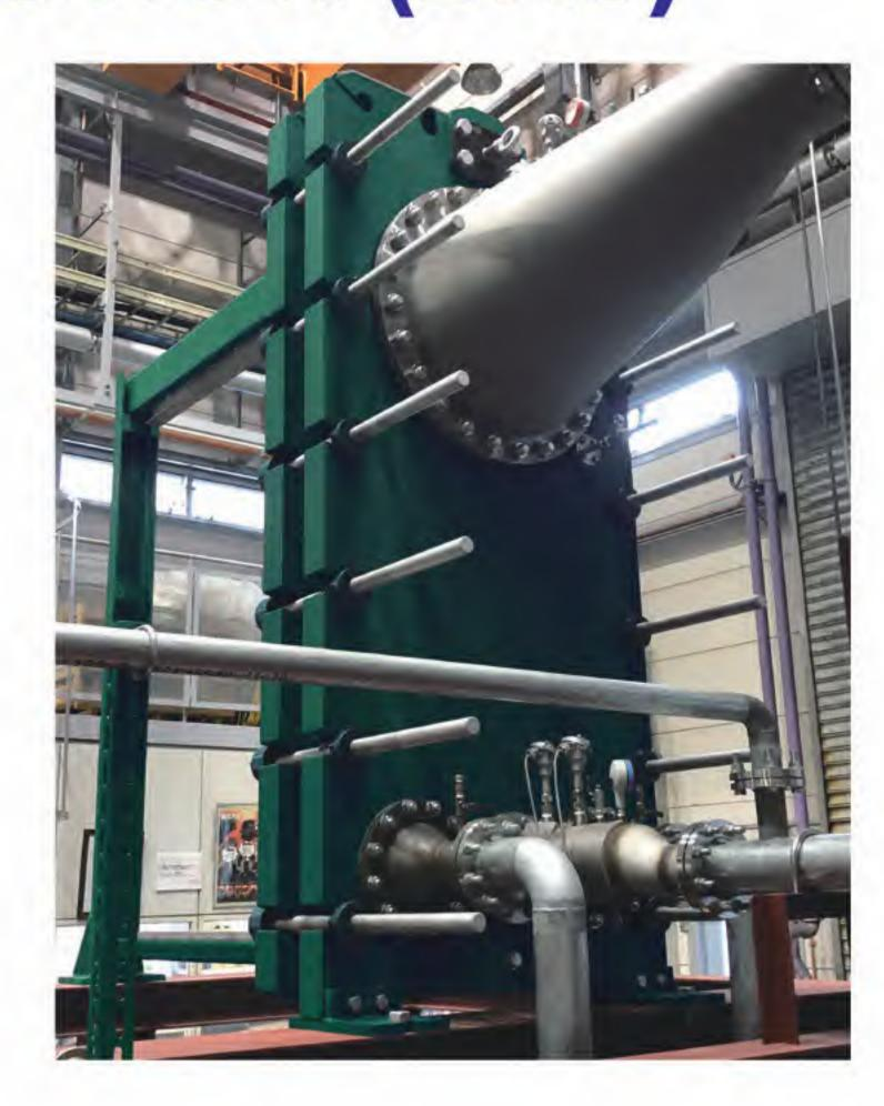
New proposal for condenser with high flow rate to save installation space
