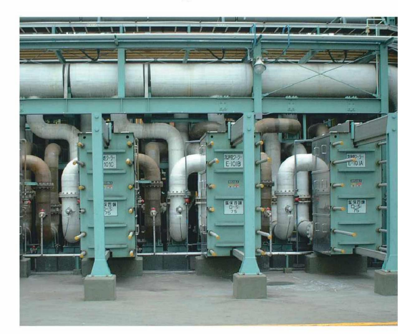
Sulfuric acid, electrolytic plating cooling
