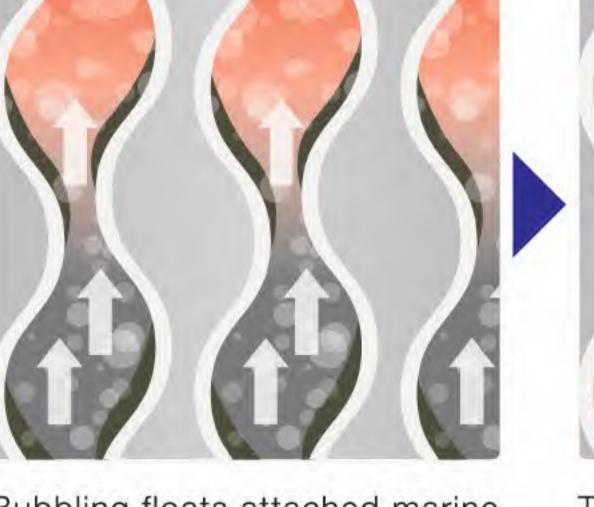
Bubbling floats attached marine organisms up to the surface.
