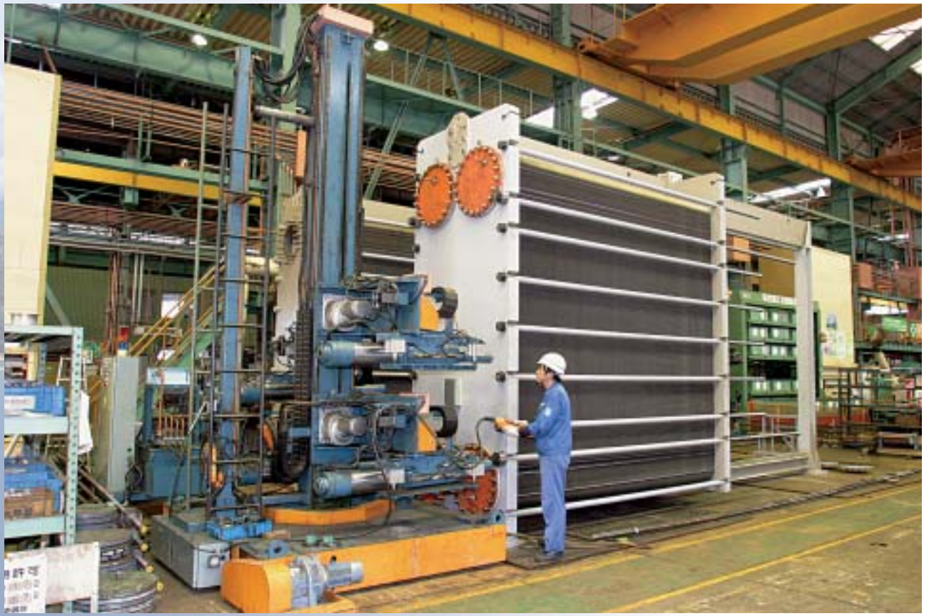
Large plate type heat exchanger being assembled by a large automatic tightening device
