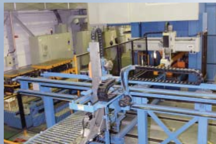
The latest 4,000-ton high-speed automatic precision pressing line
