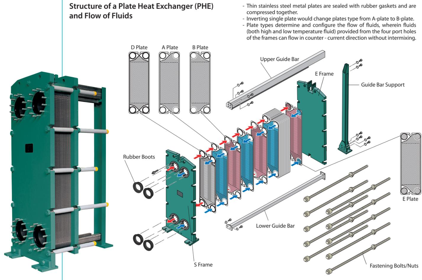
HISAKA Plate Heat Exchanger (PHE) has press-molded herringbone patterns which increases the heat transfer performance even with a reduced heat transferring area as compared to shell and tube heat exchangers. In comparison:
